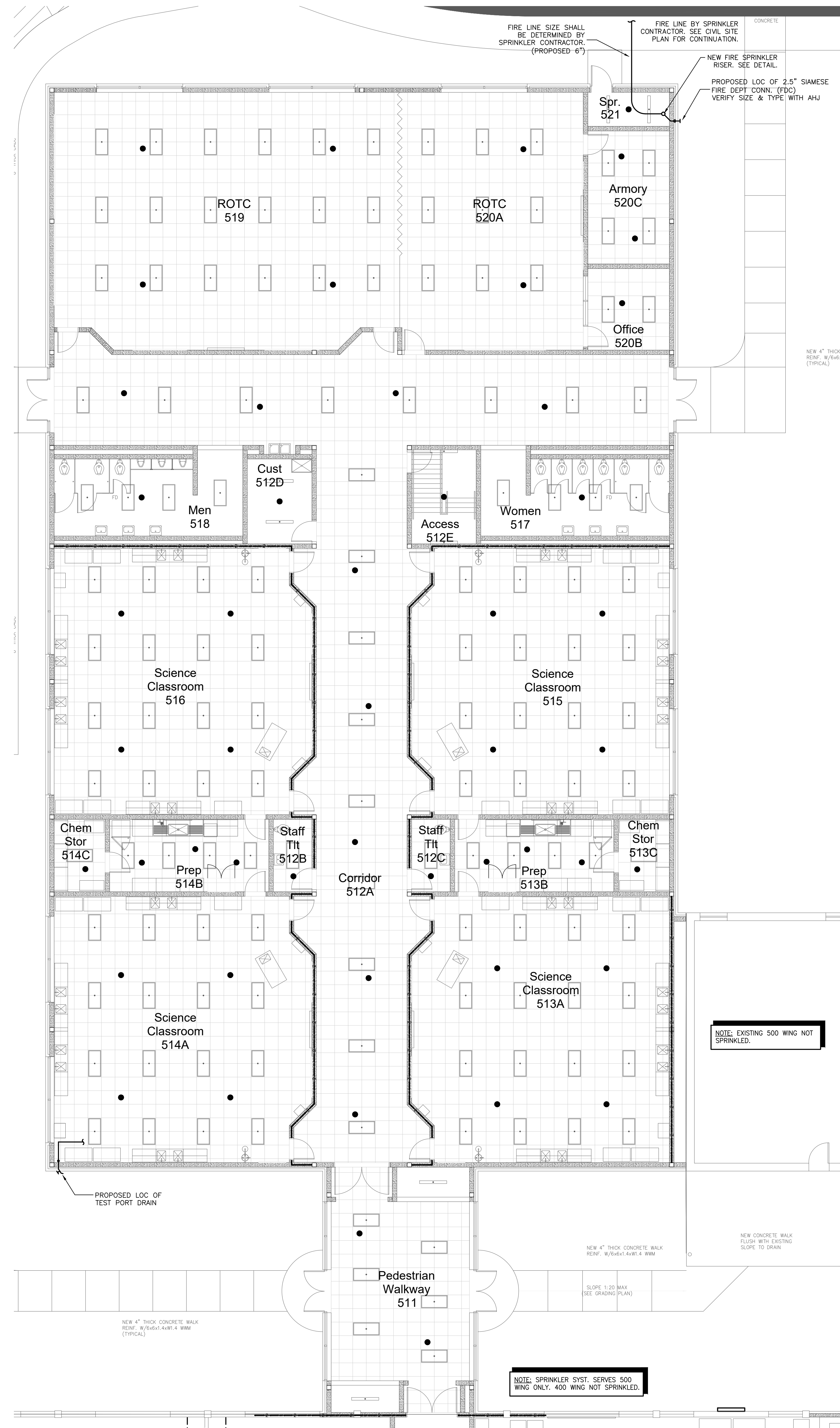
501.1 FIRE SUPPRESSION PLAN - SCIENCE ROOMS SCALE: 1/8" = 1'-0"
