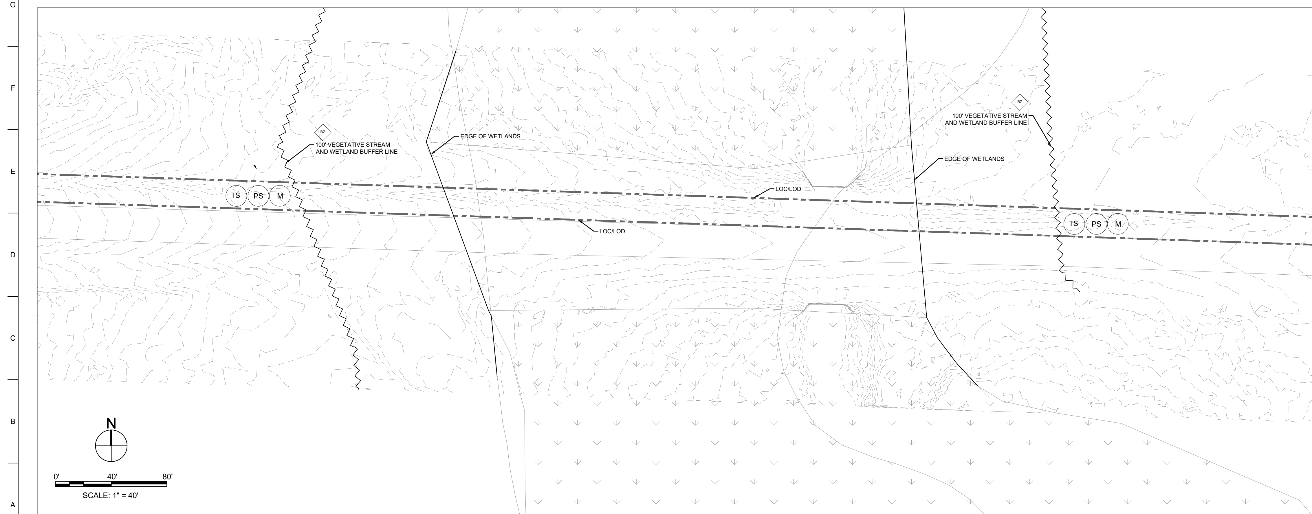
OFFSITE COMMUNICATION UTILITY PLAN DETAIL
