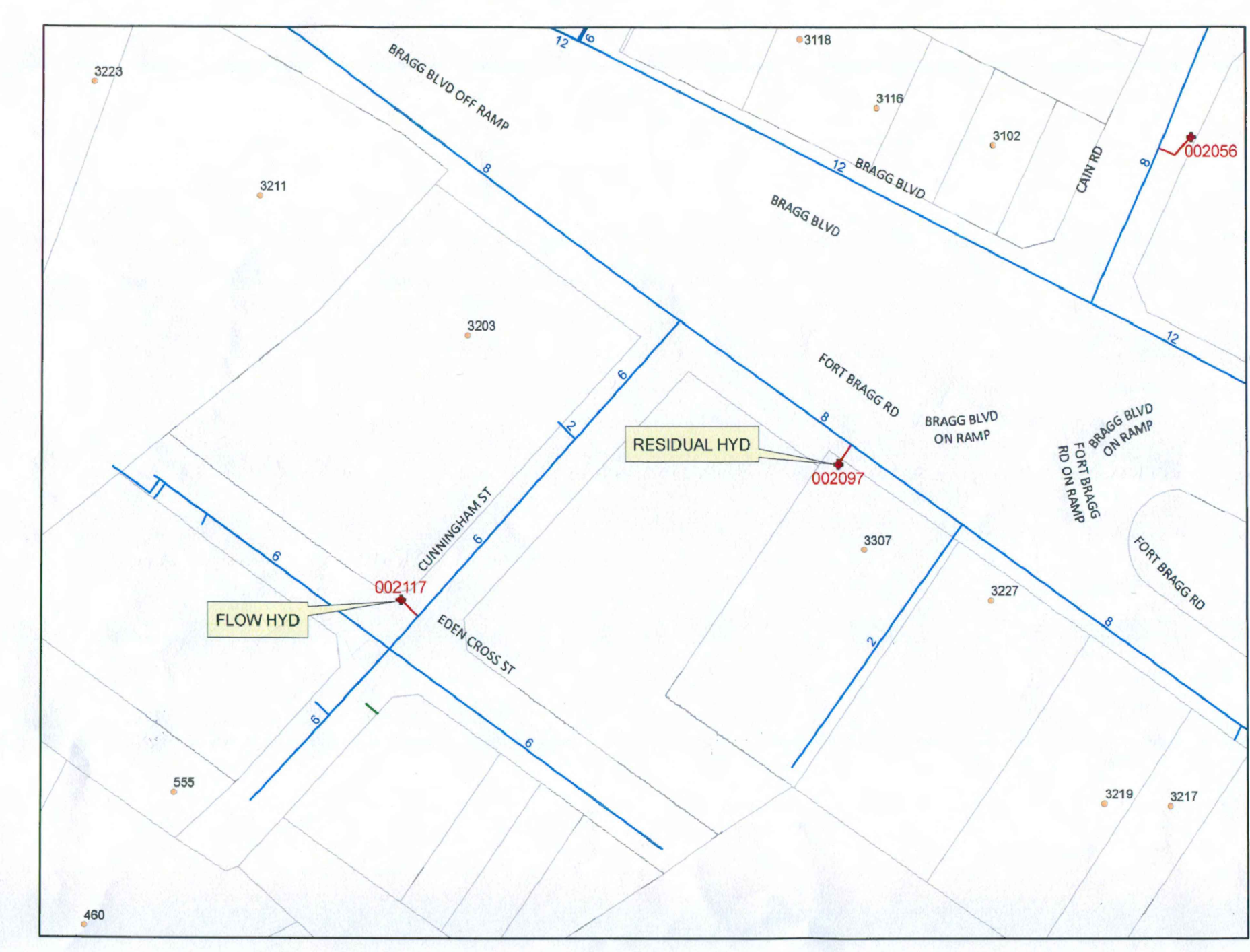
HYDRANT FLOW TEST - 3307 FORT BRAGG ROAD - 2314147
