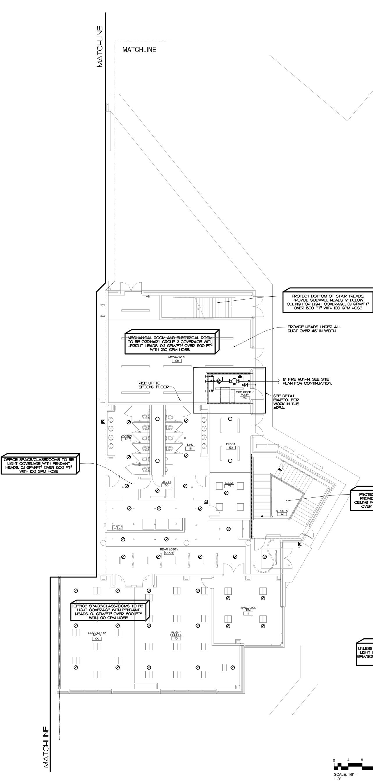
PROTECT BOTTOM OF STAIR TREADS. PROVIDE SIDEWALL HEADS 12" BELOW CEILING FOR LIGHT COVERAGE. O.I GPM/FT<sup>2</sup> OVER 1500 FT<sup>2</sup> WITH 100 GPM HOSE
