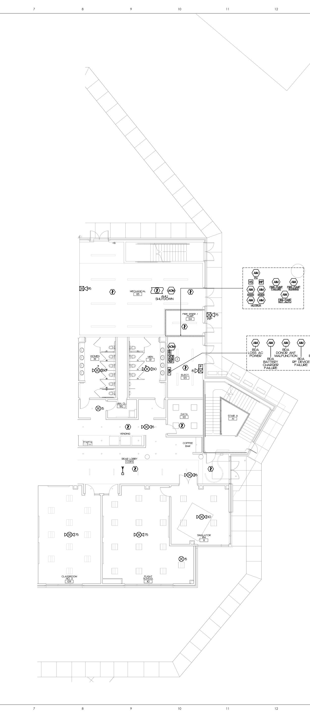
16 17 18 KEY NOTES FIELD COORDINATE FIRE ALARM CONTROL PANEL LOCATION WITH FIRE MARSHAL PRIOR TO ROUGH-IN. (2) INSTALL IF REQUIRED. SEE TI5/FA0.0 FOR DETAILS.
