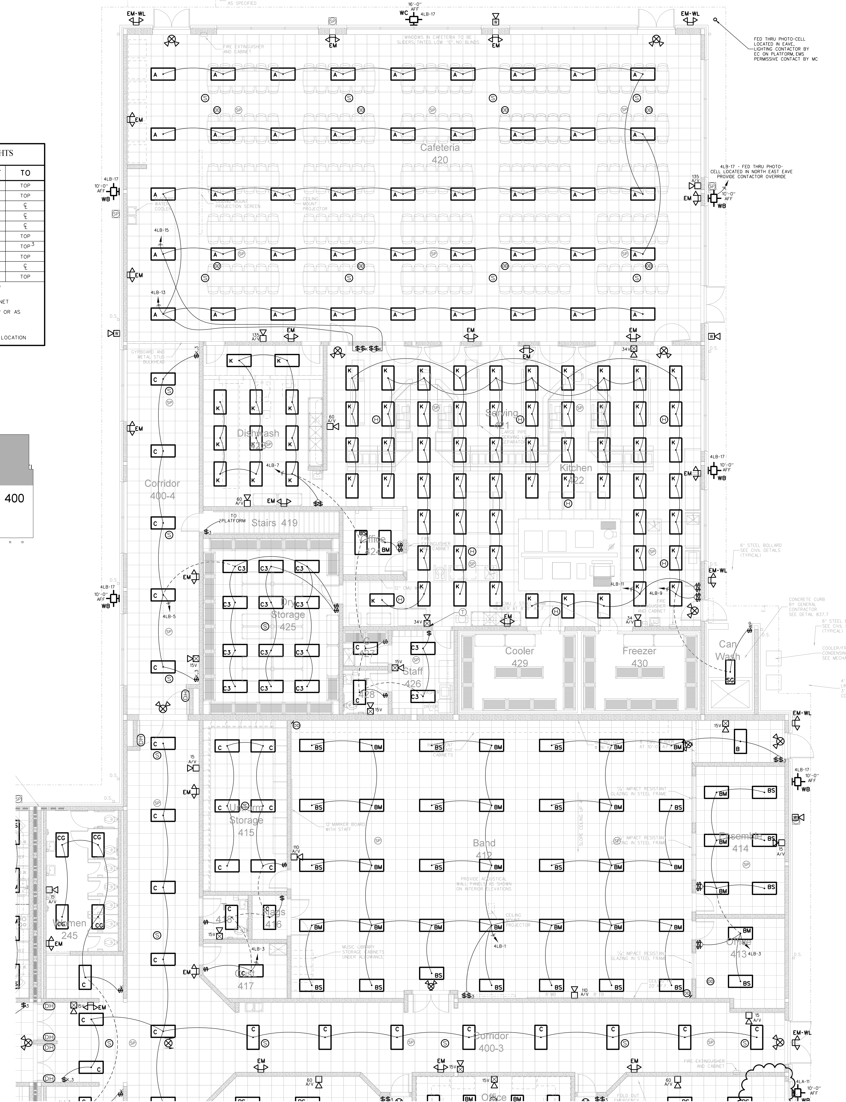
404.1 BAND/ CAFETERIA / KITCHEN LIGHTING / FIRE ALARM PLAN SCALE: 1/8" = 1'-0"
