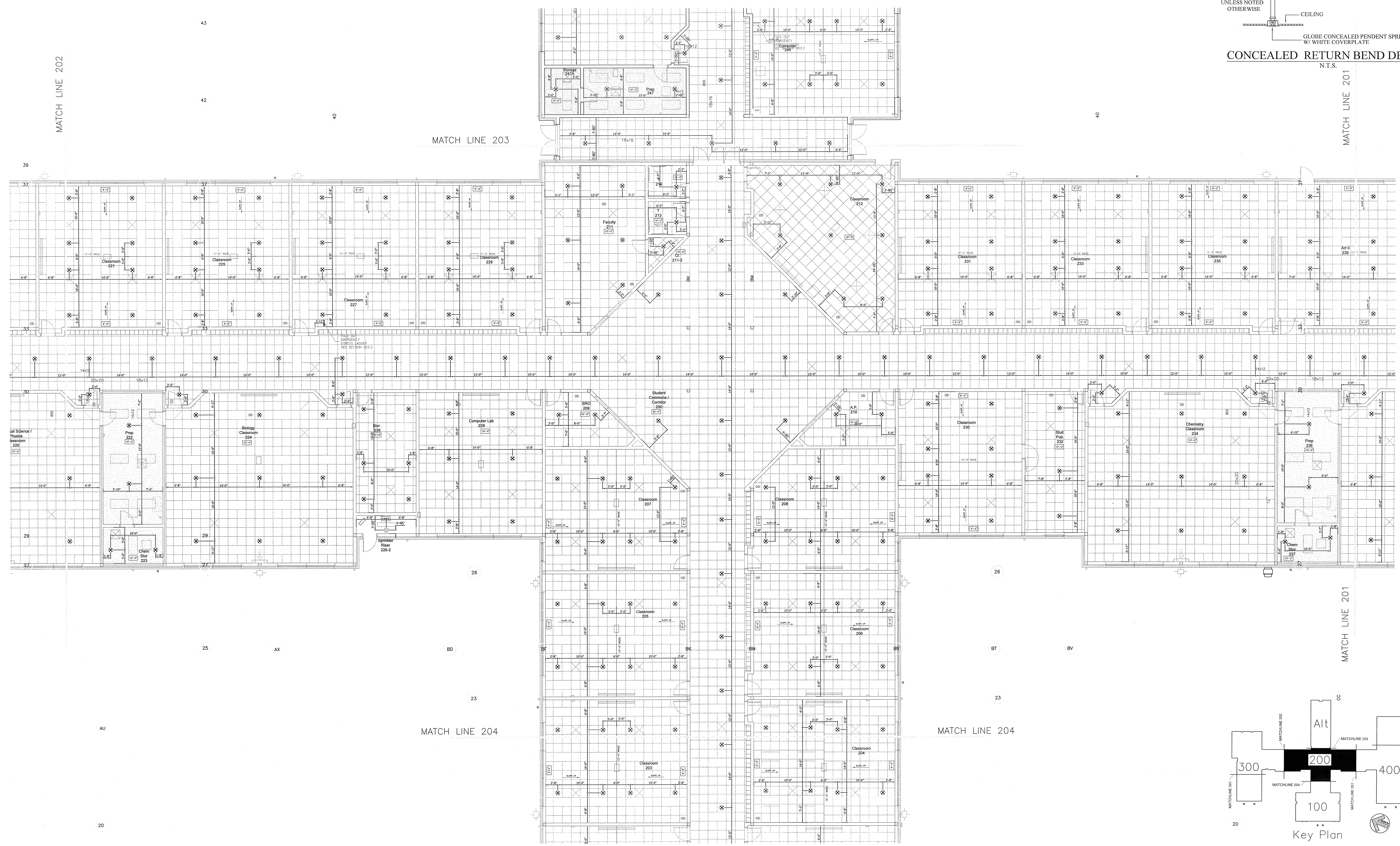
CLASSROOM 200 WING FIRE PROTECTION HEAD LAYOUT PLAN SCALE: 1/8" = 1'-0"
